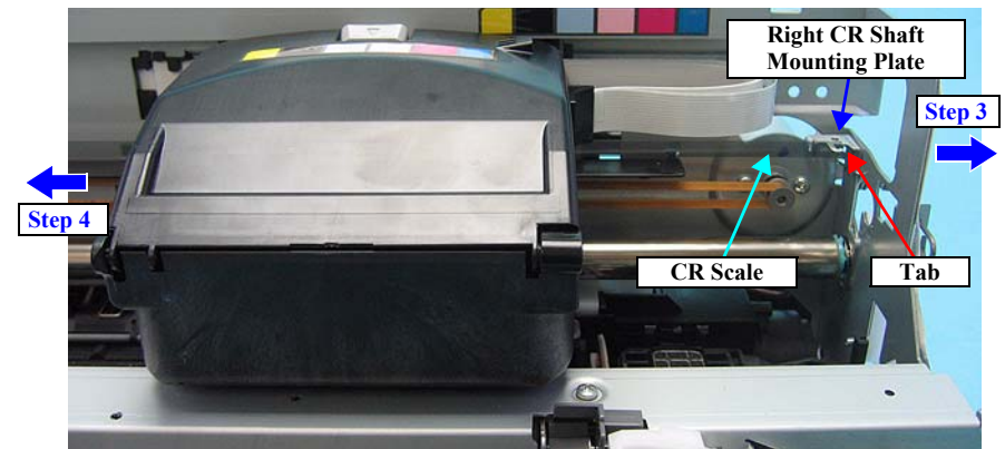
Figure 4-41. Drawing Out the CR Scale
